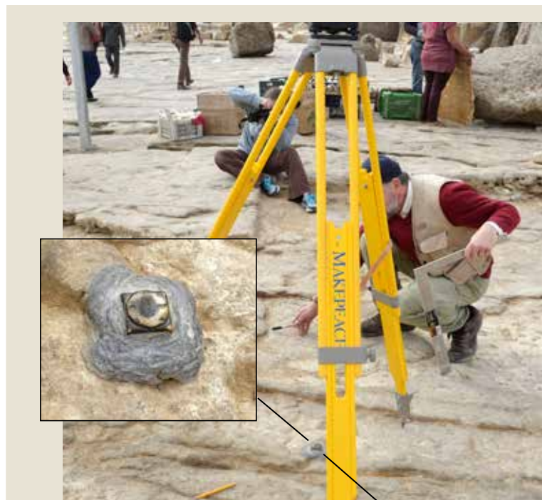
On the south side of the Great Pyramid there was no direct evidence of where the casing stones met the platform. In order to project where the casing stones once would have fallen on the platform below, Glen Dash measures the top outer edge of the casing stones, assisted by Rebecca Dash. Photo by Mark Lehner.
